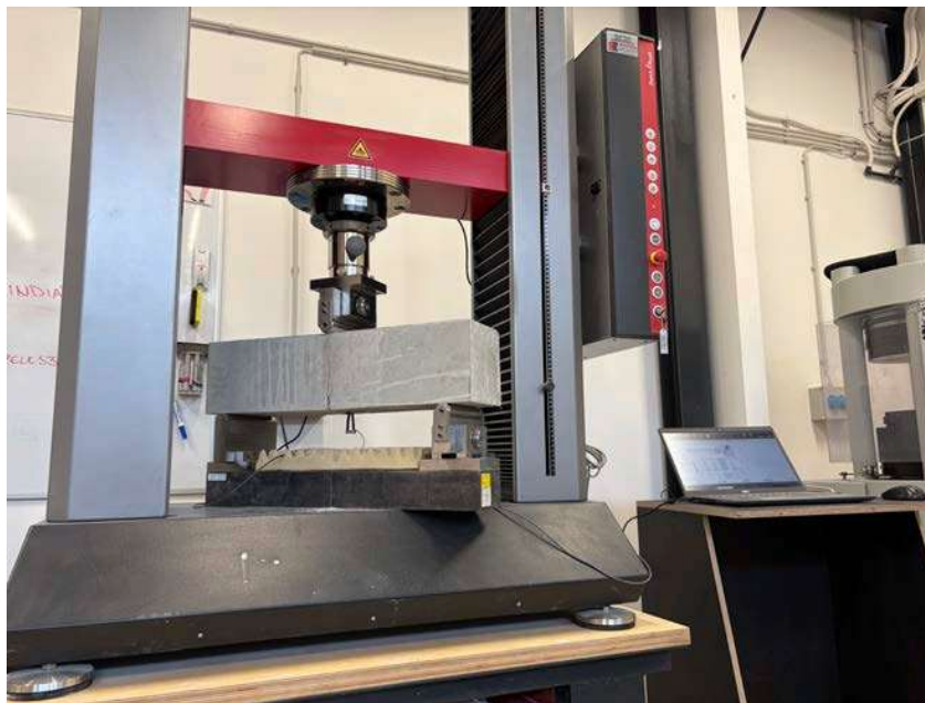
Figure 1. 3PBBT according to EN 14651 in JKP STATIC Concrete Laboratory
